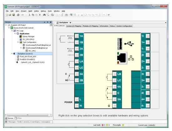
A view of the terminal block is shown. Click in any of the grey selection boxes to show a list of available input or output types. The list of available I/O is opened under the **Backplane** folder.
