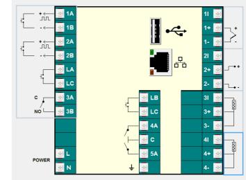
A diagrammatic representation of the I/O type is shown connected to the relevant terminal. Note that terminals with an I suffix (capital letter 'i') act as a current source for resistance measurements. In the example shown:
