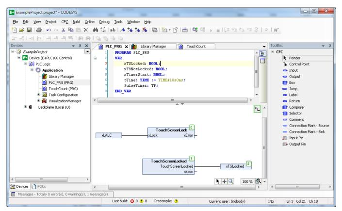
To produce the TouchScreenLock function block, Drag a 'Box' to the screen. Begin to type 'E\_SL' (Eurotherm Screen Lock) and select this from the pop up. Then begin to type '.' and select 'TouchScreenLock'.
