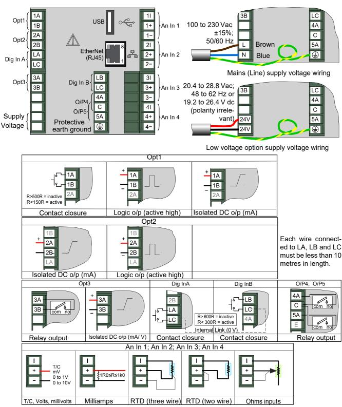
For thermocouples use the correct type of compensating cable and maintain polarity throughout.
