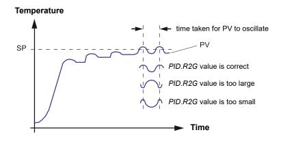
Figure 6.2.4d Relative Cool Gain waveform tuning
