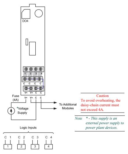
Figure DO4-1 Four Channel Digital Output Module Terminal Connections
