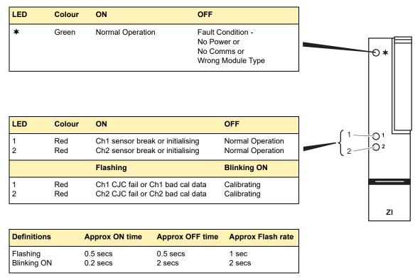
Figure ZI-4 Two Channel Zirconia Input Status Indication
