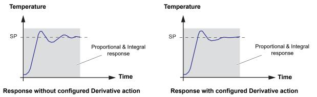
Figure 6.2.3c Derivative Time (Td) configuration
