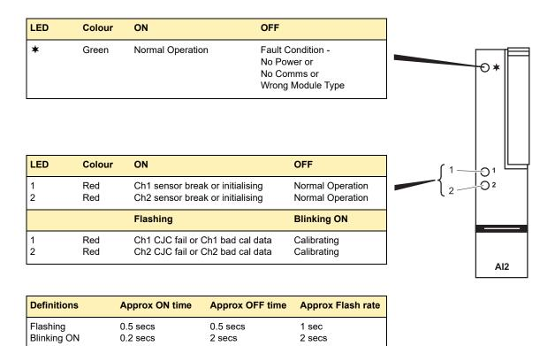
Figure Al2-8 Two Channel Analogue Input Status Indication
