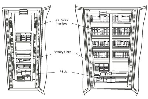
Figure 1.4.2a Typical installations
