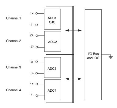
Figure Al4-2 Isolation Diagram
