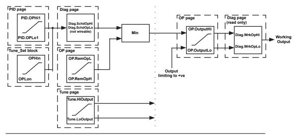
Note Each OPHin and OPLon are derived from a Tune\_set block identified by the n, where n equals the PID set number.
