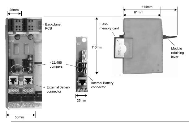
Note The dimensions shown for the Duplex Terminal Unit also apply to the Profibus Terminal Unit.
