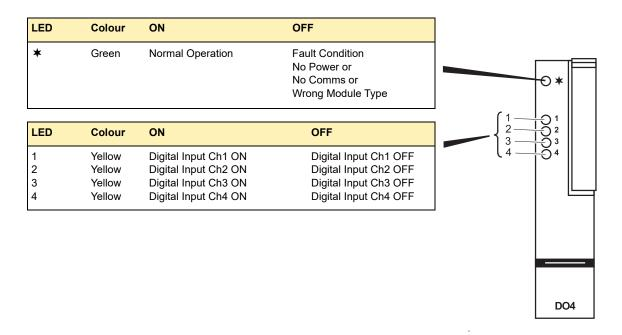
Figure DI8-5 Four Channel Digital Output Module Status Indication
