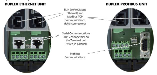
Figure 2.5.1a Communication Ports
