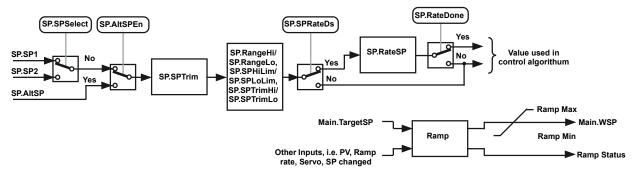
Figure 6.2.5a SetPoint, SP, page block diagram
