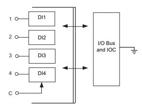
Figure DI4-2 Isolation Diagram
