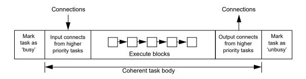
Figure 7.2.3b User task block server operation
