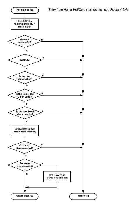
Figure 4.2.4b Hot or Hot/Cold start flowchart
