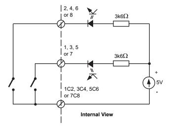
Figure DI8-4 Contact Closure Input Equivalent Circuit
