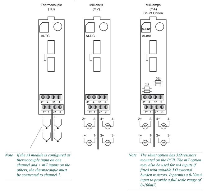
Figure Al4-1 Terminal connections
