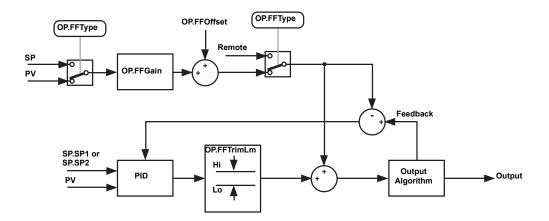
Figure 6.2.6b FeedForward block diagram
