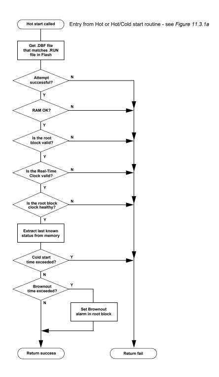
Figure 11.3.1b Hot/Cold Start routine flowchart - simplified
