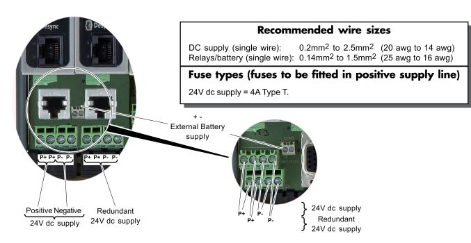
Figure 2.5.3 DC and relay connection details
