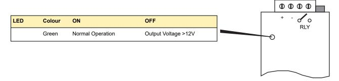
Figure D1.6 2500P Power Supply Status Indication
