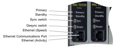
Figure 3.3 Changeover LEDs and switches
