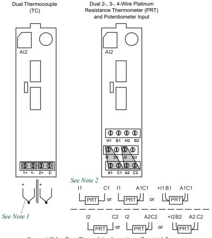
Figure Al2-1a Two Channel Analogue Input Terminal Connections
