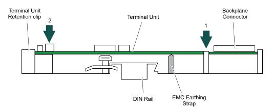
Figure 2.3.3 Fitting a Terminal Unit (Side View)
