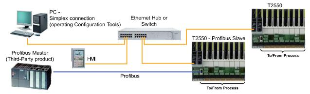
Figure 2.5a Typical overall Simplex connection diagram
