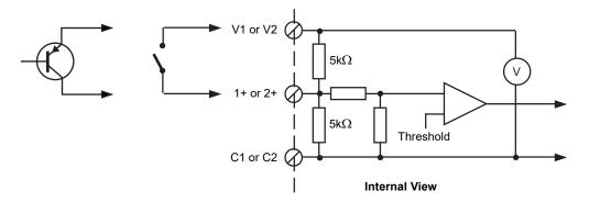
Figure FI2-6 Contact Inputs (PNP) or Volt-Free
