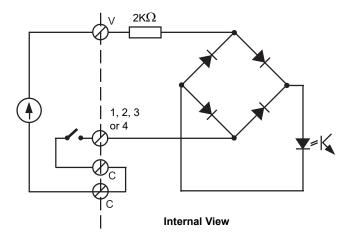
Figure DI4-4 Contact Closure Input Equivalent Circuit
