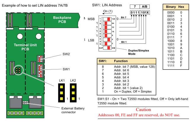
Figure 2.4.2b Location of Duplex Terminal Unit switches
