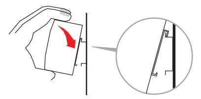
3. Push downwards until stopped, then push at the lower front edge to lock.
