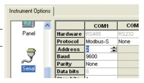
■ The Modbus registers must be set at the Offsets shown.
