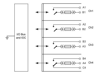
Figure RLY4-2a Isolation Diagram - Fused Option
