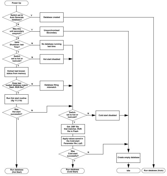
Figure 11.3.1a Power-up routine flowchart - simplified
