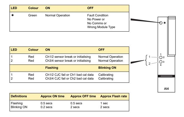
Figure Al4-6 Four Channel Analogue Input Status Indication
