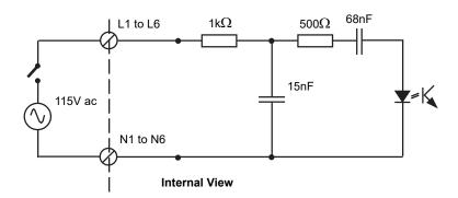
Figure DI6-4 115V ac Digital Input Equivalent Circuit
