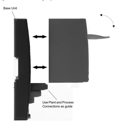
Figure 2.3.4 Module fitting/removal
