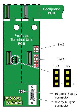
Figure 2.4.2d Location of Profibus Duplex Terminal Unit switches
