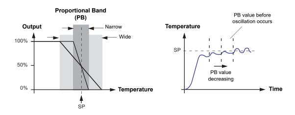
Figure 6.2.3a Proportional Band (PB) configuration
