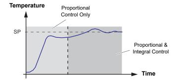
Figure 6.2.3b Proportional Band (PB) configuration
