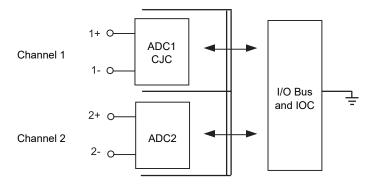
Figure Al2-2 Isolation Diagram
