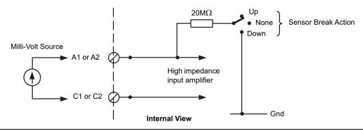
Note When an input is configured as mV or V, the input circuit is selected based on the configured range parameters HR\_in and LR\_in. See section D2.2 - Terminal Connections. When InType is set to Zirconia, the range is fixed at 0-1800mV.
