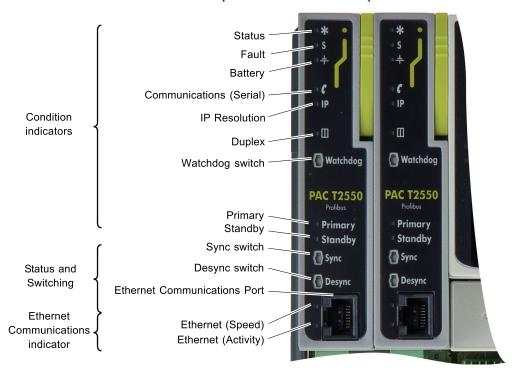
Figure 11.2.1 Front panel layout (Redundant Configuration)
