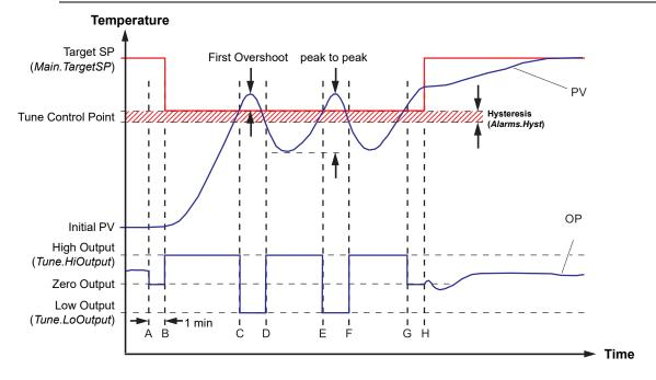
Figure 6.2.4a Tuning from below SP - Heat/Cool control loop
