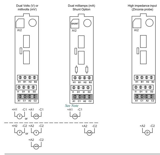
*Note* The Shunt option has  $5\Omega$  resistors mounted on the rear of the PCB.
