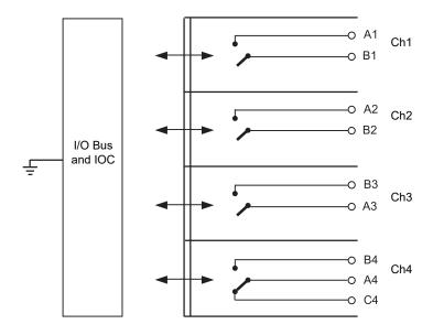
Figure RLY4-2b Isolation Diagram - Unfused Option
