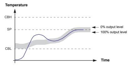
Figure 6.2.3d High and Low Cutback (CBH and CBL) configuration
