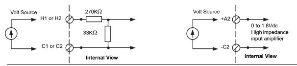
Note When an input is configured as mV or V, the input circuit is selected based on the configured range parameters HR\_in and LR\_in. See section D2.2 - Terminal Connections. When InType is set to Zirconia, the range is fixed at 0-1800mV.
