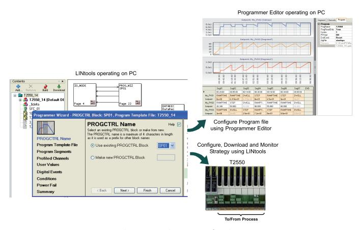
Figure 10.2 Setpoint Program Configuration
