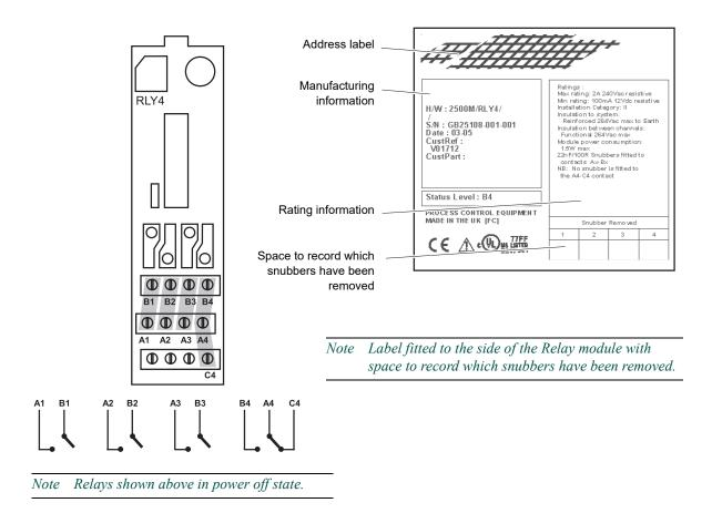
Figure RLY4-1 Relay Module Terminal Connections
