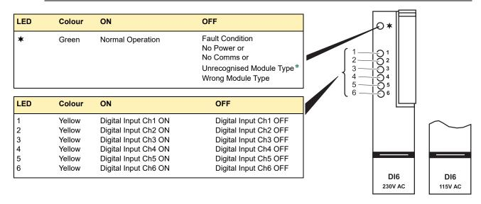
Figure DI6-5 Six Channel AC Digital Input Module Status Indication
