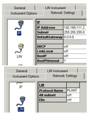
However, if the instrument is to have a fixed IP Address, i.e. 192.168.111.2, and use the LIN Protocol Name, 'PLANT', the Instrument Properties dialog must be used to modify these parameters.
