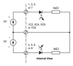
Figure DI8-3 Logic Input Equivalent Circuit
