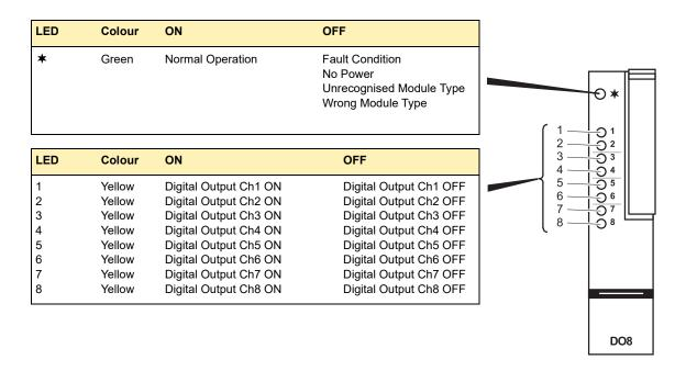
Figure DO8-4 Eight Channel Digital Output Module Status Indication
