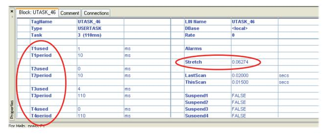
In order to ensure smooth running, the amount of time used in executing all the blocks in all the tasks must not exceed 90% of the time available, otherwise there is insufficient time for non-task events (e.g. ftp transfers) to take place.
