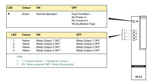
Figure RLY4-3 Relay Module Status Indication
