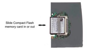
Figure 12.2.1 Replacing the Compact Flash Memory Card
