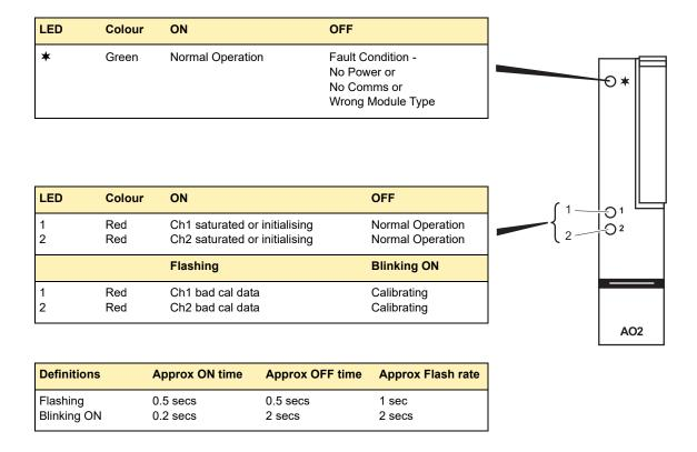
Figure AO2-5 Two Channel Analogue Output Status Indication
