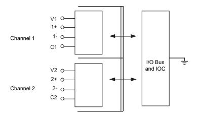
Figure FI2-2 Isolation Diagram
