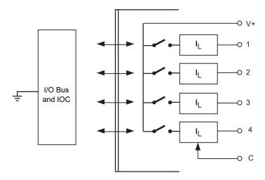
*Note I*, *indicates the current-limit mechanism.*
