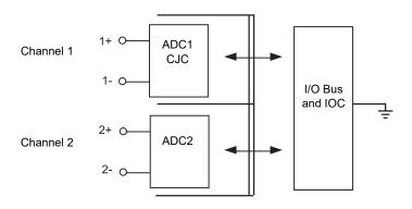
Figure ZI-2 Isolation Diagram
