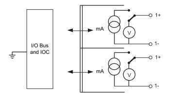
Figure AO2-2 Isolation Diagram
