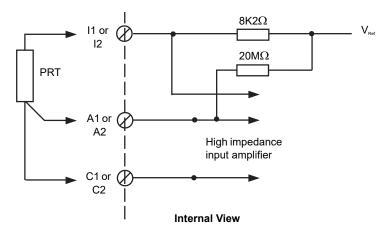
Figure Al2-4 3-Wire PRT Input
