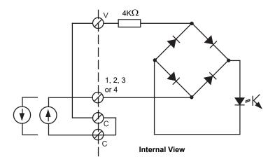
Figure DI4-3 Logic Input Equivalent Circuit
