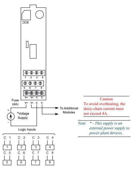
Figure DO8-1 Eight Channel Digital Output Module Terminal Connections
