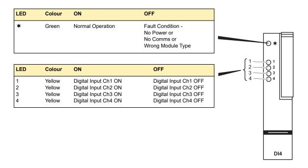
Figure DI4-5 Four Channel Digital Input Module Status Indication
