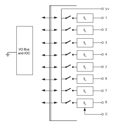
Note  $I_L$  indicates the current-limit mechanism.
