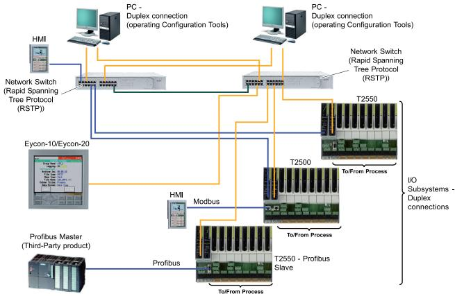
Figure 2.5b Typical overall Duplex connection diagram
