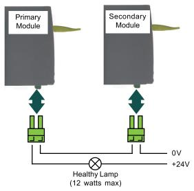
Figure 2.5.5b Watchdog Relay - Series Wiring
