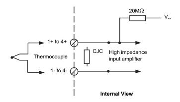
Figure Al4-3 Thermocouple Input
