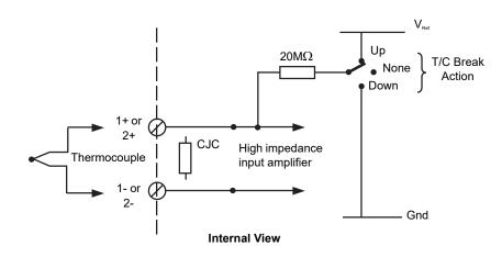
Figure AI2-3 Thermocouple Input
