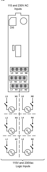
Figure DI6-1 Six Channel AC Digital Input Module Terminal Connections
