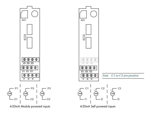
Figure Al3-1 Three Channel Analogue Input Terminal Connections
