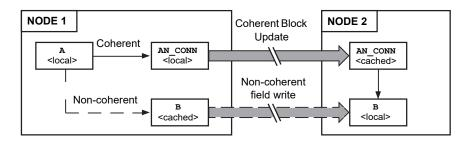
Figure 7.4 Coherent and non-coherent data flow across network
