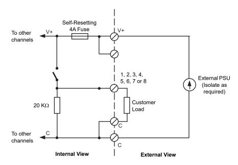
Figure DO8-3 Voltage (24V) Switch Output Equivalent Circuit
