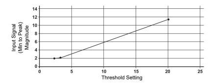
Note To allow for Hysteresis and Threshold accuracy with temperatures and between modules that have been swapped, the input signal MUST have sufficient amplitude. Use this graph as a guide to the size of signal for a given Threshold setting.
