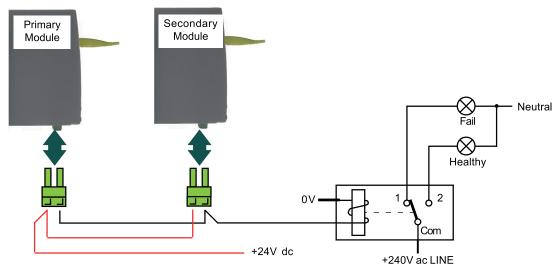
Figure 2.5.5c Watchdog Relay - Parallel Wiring
