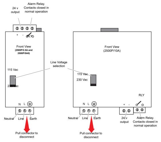
Figure D1.5 2500P Power Supply Terminal Connections
