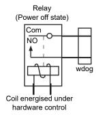
Figure 2.5.5a Relay Wiring
