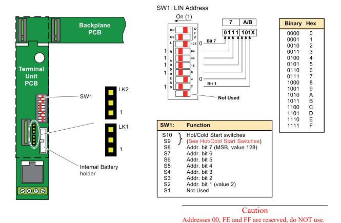
Figure 2.4.2a Location of Simplex Terminal Unit Switches
