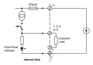
Figure DO4-3 Logic Output Equivalent Circuit
