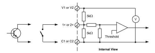
Figure FI2-7 Contact Inputs (NPN) or Volt-Free
