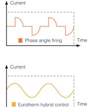
Analog thyristor controllers waste energy by drawing more power from the supply than is required by the heater, due to harmonic generation at most setpoint levels.
