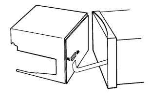
Figure 2 Flexi-cable removal
