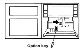
Figure 1 Option key and jacking bolt locations
