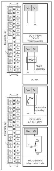
4- / 8-channel analogue output board (typical outputs)
