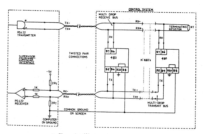
Figure 1 RS422 Data Bus Connections
