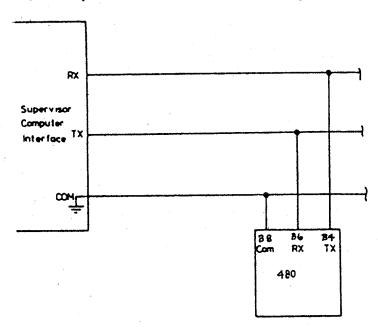
Figure 2 RS232 Data Bus Connections
