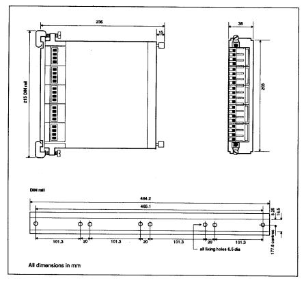
The 483 load sequencing controller is supplied complete with base plate, for mounting on to parallel DIN rails, or direct on to a control panel backplate. The unit should be mounted in a vertical plane. If fitting to DIN rails, release the top and bottom fixing screws 2 turns, drop onto rails, slide laterally into correct position and tighten up screws.
