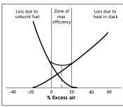
In actual practice, gas, oil, coal burning and other systems do not do a perfect job of mixing the fuel and air under the best achievable conditions. Additionally, complete mixing may be a lengthy process. Figure 1 shows that in order to ensure complete combustion and reduce heat loss, excess air has to be kept within a suitable range.
