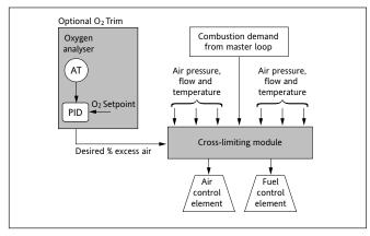
Figure 3 Cross-limiting combustion control with 06 trim
