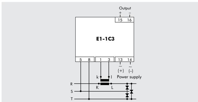
Three phase three wire balanced load
