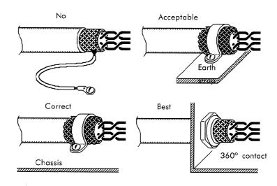
When connection is made by a screw connector block, the length of the pigtail must be minimised. This type of connection is preferably to be avoided.
