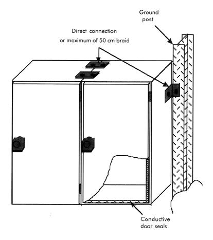
Within the interior of the cabinet, creation of a ground mesh is achieved by interconnecting all metal parts.
