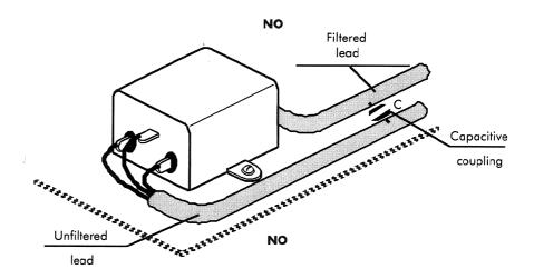
• Loose wiring- keep input and output cables close against the metal chassis in order to prevent them picking up airborne interference
