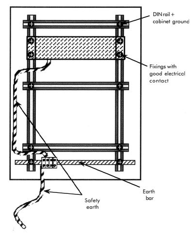
Equipment mounted on a DIN rail will often be linked directly through the mechanical mounting. This should be checked.
