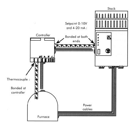
Control signals and low level analogue signals
