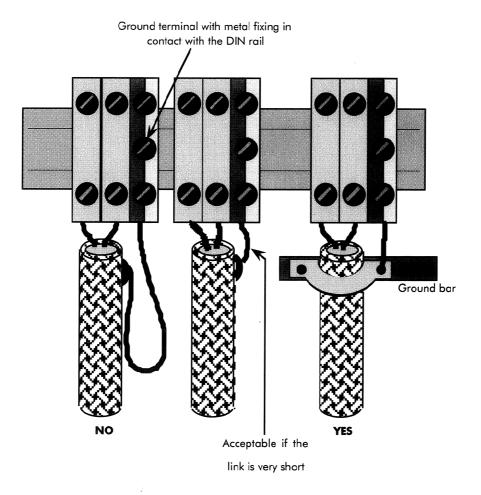
In the case of wiring using a connector, the mechanical coupling of the connection must achieve continuity throughout its circumference between the screen of the cable and the case of the equipment.
