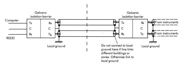
Use of isolating line drivers for long distance digital transmission has safety implications. If ends are located in this case break the ground connections at the isolators in the building or zone remote from the computer.
