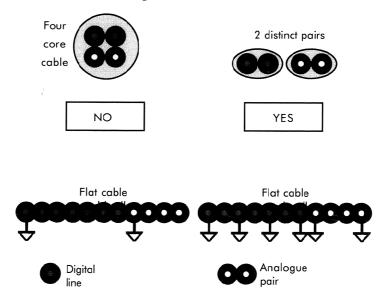
If possible, with flat ribbon cables a ground lead should be alternated with a signal lead in order to limit crosstalk.
