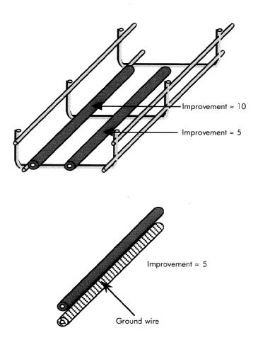
These improvements are only possible if both end points of the cable trays are connected to ground. To obtain the required results, the cable tray must have electrical continuity from end to end and be directly connected to the ground of the cabinet. One should make this coupling using a metal strap or foil since a thin ground wire 10cm long reduces the effectiveness by at the very least a factor of 5.
