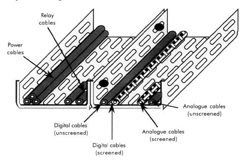
In the case when a single cable tray is used, the unscreened cables must be put in the 'shadow' area and screened cables in the centre of the tray.
