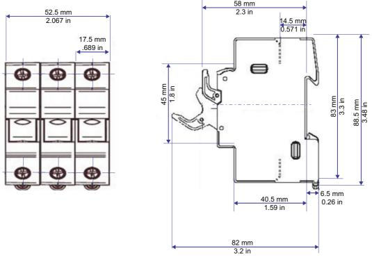
Figure 150 Fuse holder dimensions: US103 (10x38mm)
