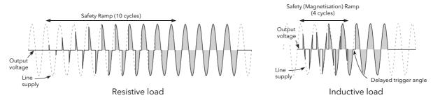
Figure 95 Safety ramp (burst firing) examples
