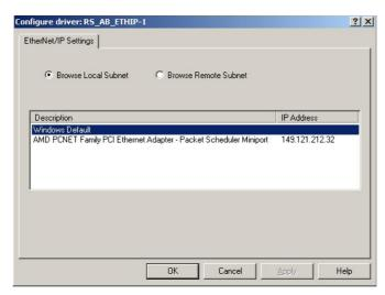
Figure 39 RSLinx Classic configure driver Ethernet/IP settings Now you are in a position to browse your network and locate EPack.
