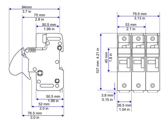
Figure 152 Fuse holder dimensions: US143 (14x51mm)
