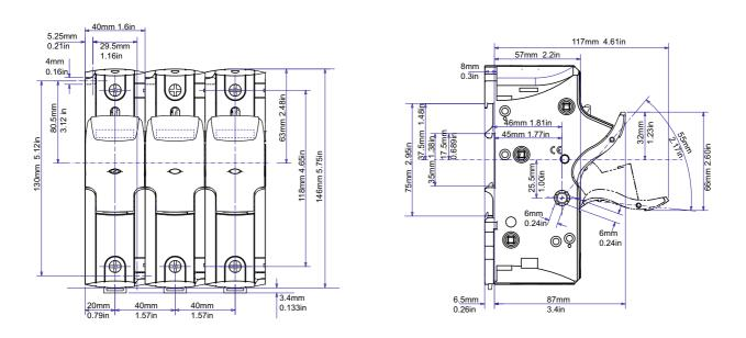
Figure 154 Fuse holder dimensions: US273 (27x60mm)
