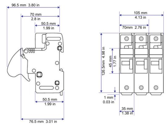
Figure 153 Fuse holder dimensions: US223 (22x58mm)
