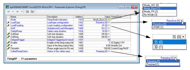
Figure 94 iTools configuration firing output page
