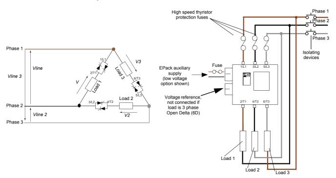
Figure 11 3 phase Open Delta wiring scheme/load configuration
