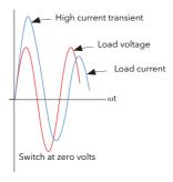
Figure 97 Delayed trigger definition
