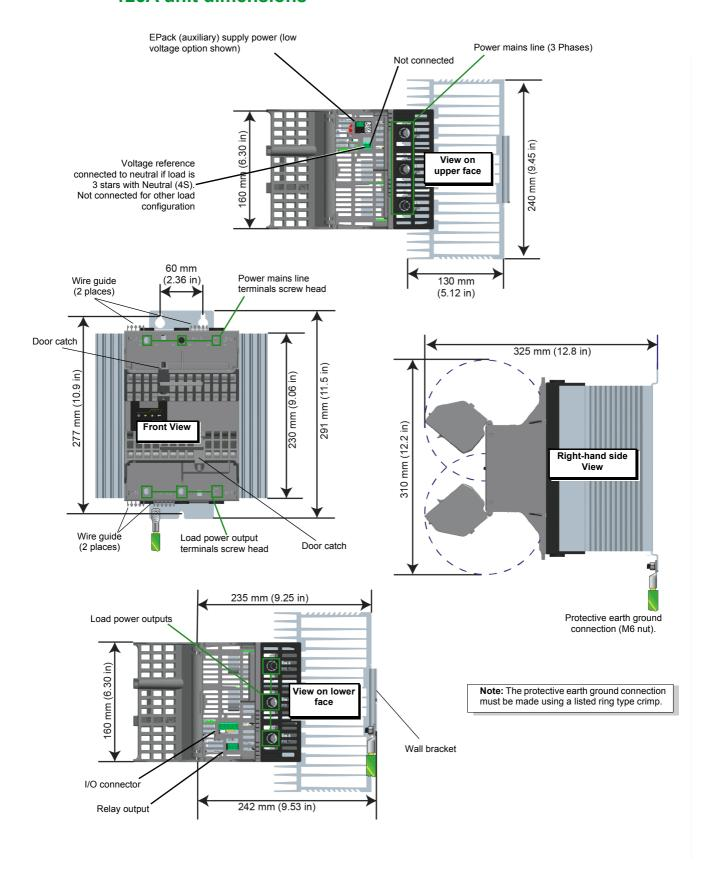
Figure 7 Mechanical installation details (125A units) (Doors open).
