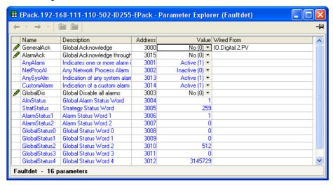
Figure 93 Fault detection menu page
