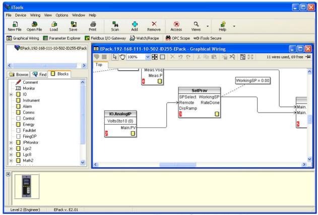
Figure 133 Graphical wiring Editor
