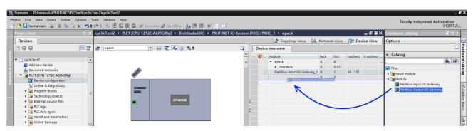
Figure 51 "Drag and Drop" I/O Modules
