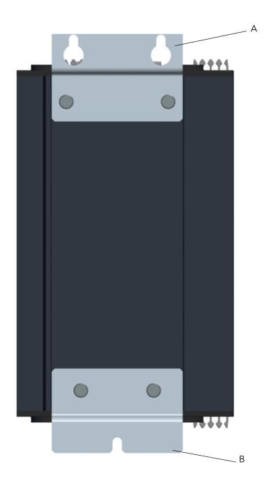
Figure 2 Bulkhead mounting 80A/100A unit shown (125A similar)
