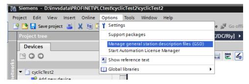
Figure 50 Loading the EPack GSDML file into STEP7
