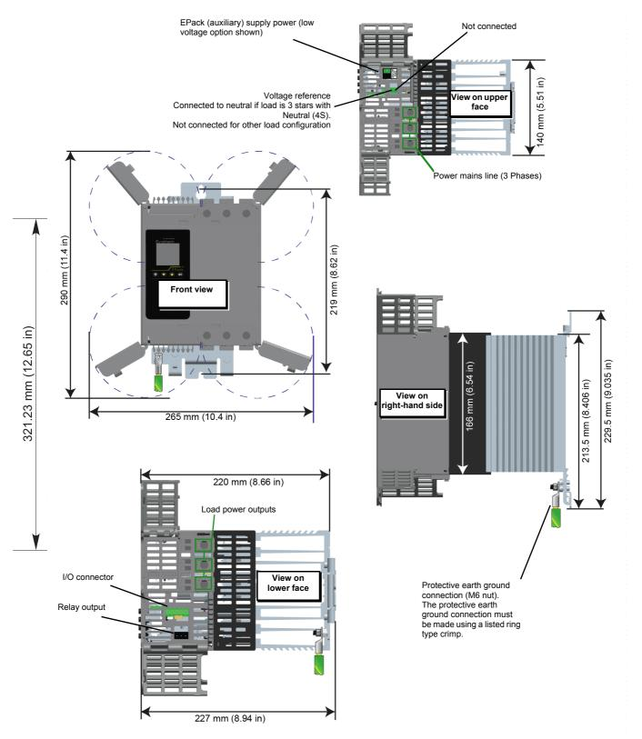
Figure 5 Mechanical installation details (40A to 63A units)
