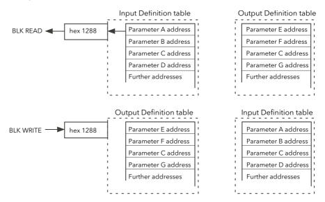
Figure 148 Block read and block write (note 3)
