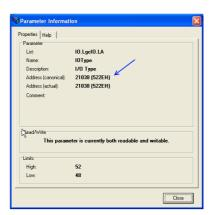
Figure 53 Parameter Access using the Graphical Wiring Editor From this address, use the following conversion to get the PROFINET way of addressing a parameter:
