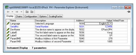
Figure 105 Top level instrument configuration page
