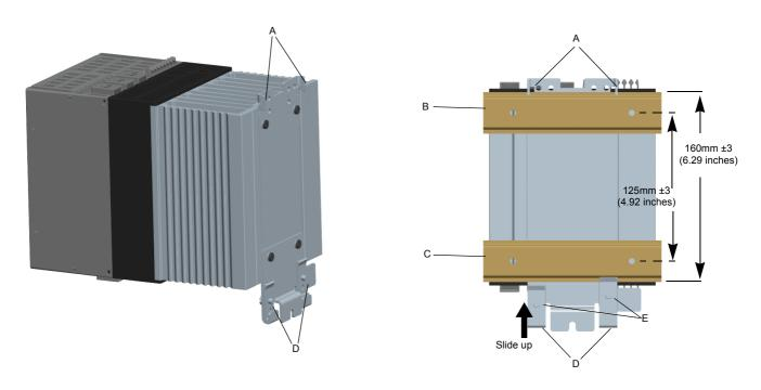
Figure 3 DIN rail mounting (32A unit shown; 63A units similar)
