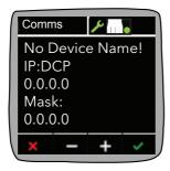
Figure 45 EPack 'Comms' screen display 'as-delivered' (Device Name = "", IP Configuration = Null).
