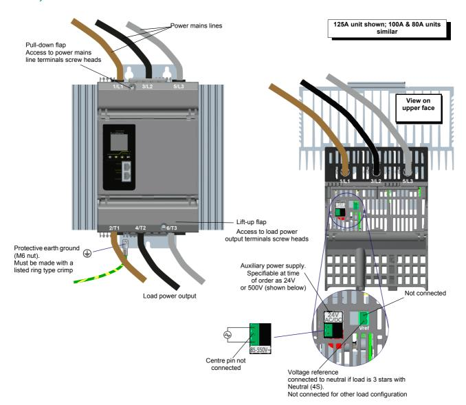
Figure 9 Supply power and Load connection details (80A to 125A units) (125A displayed).
