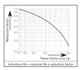
Figure 159 Relay derating curves
