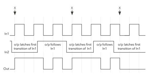
When In2 goes low, Out follows the next positive or negative transition of In1 (points 'X') and latches at this value until In2 goes high. When In2 is high, Out follows In1.
