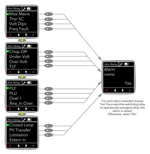
Figure 69 Alarm Relay menu
