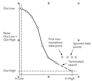
Figure 117 How an Inverted Curve will Terminate its search when it detects non-monatonic data
