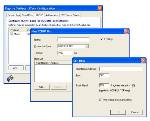
Figure 131 Adding a new Ethernet port
