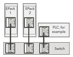
Figure 43 PROFINET Wiring - Multiple controllers
