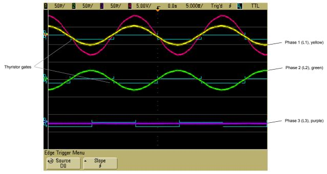
Figure 99 Waveform, unbalanced load (L3 load open circuit), ULM option on, automatically balances thyristor gates and remaining phases 1 and 2.
