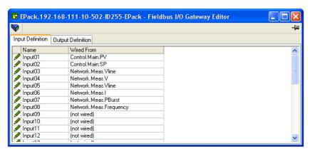
Figure 146 Typical Fieldbus Gateway Parameter list
