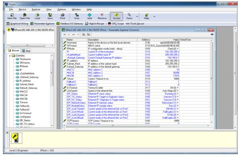
Figure 42 iTools - Ethernet Communications Parameter
