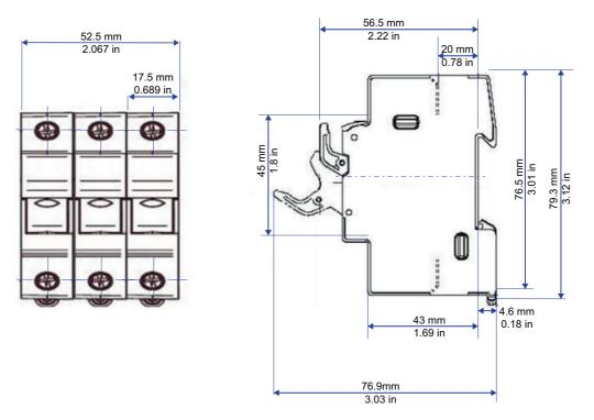
Figure 151 Fuse holder dimensions: CUS103 (10x38mm)
