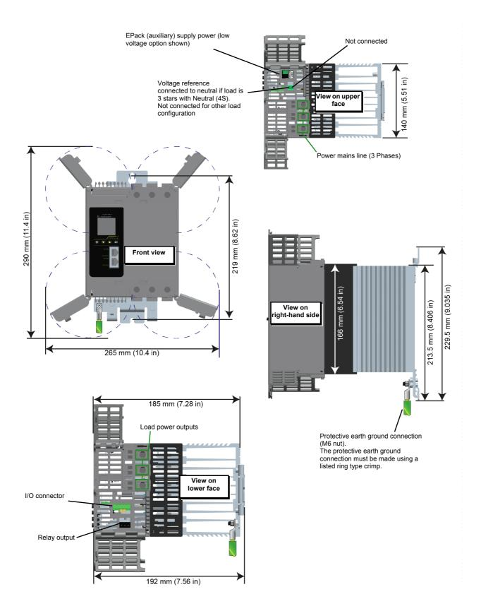
Figure 4 Mechanical installation details (16A to 32A units)
