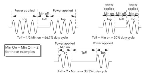
Figure 21 Burst variable firing
