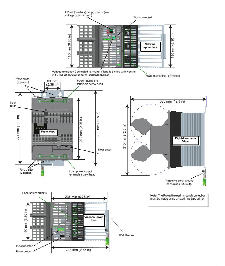
Figure 6 Mechanical installation details (80A to 100A units) (doors open).
