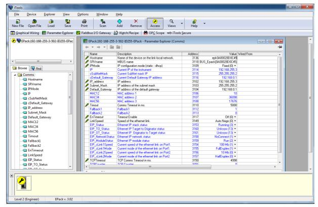
Figure 26 Ethernet/IP User Comms configuration parameters
