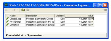
Figure 86 Control Alarm latching page
