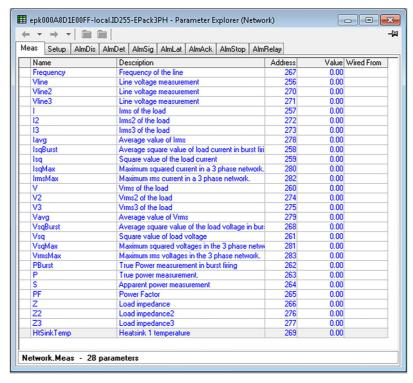
Figure 121 Network, Meas configuration panel
