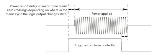
Figure 19 Logic firing mode
