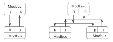
Figure 41 Single Serial Link and Multi Drop Serial Link
