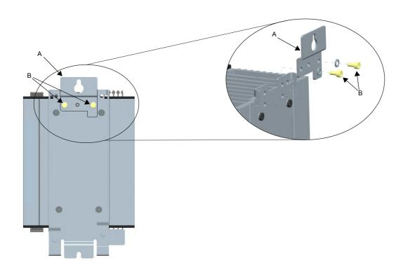
Figure 1 Fitting upper bulkhead mounting bracket (32A unit shown; 63A units similar)
