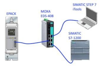
Figure 44 Configuration Tool Connections
