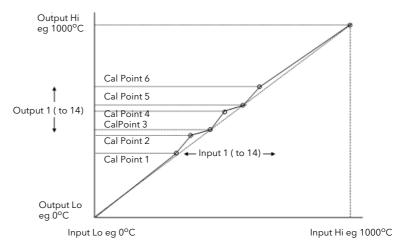
Figure 118 Compensation for Sensor Discontinuities
