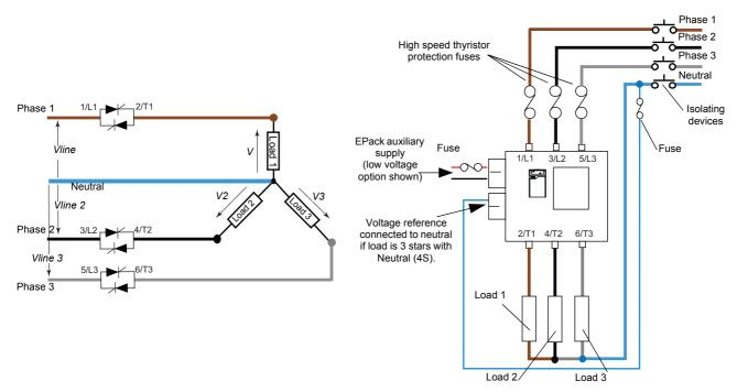
Figure 12 3 phase Star with Neutral wiring scheme/load configuration
