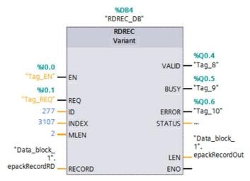
Figure 54 Reading one EPack parameter, using RDREC function block of STEP 7
