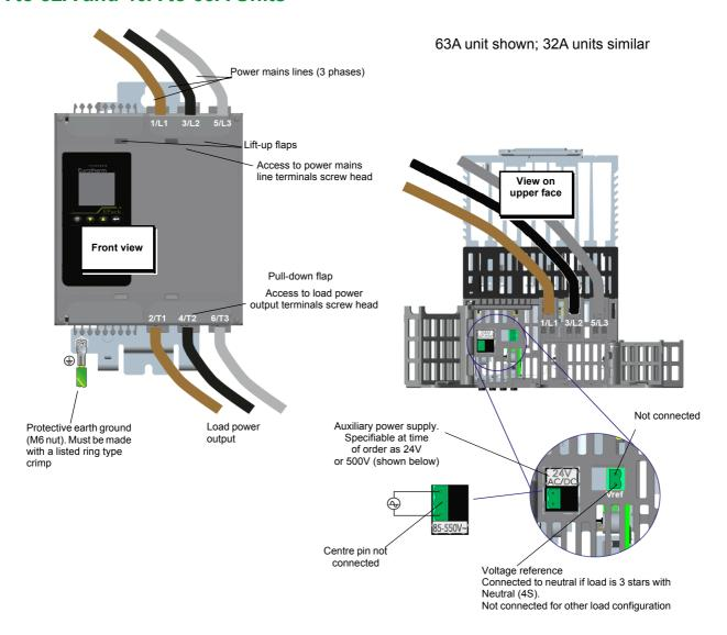
Figure 8 Supply power and Load connection details (16A to 63A units)
