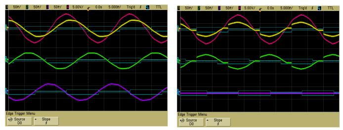
Figure 98 Waveforms; balanced load left, unbalanced load right (ULM off)
