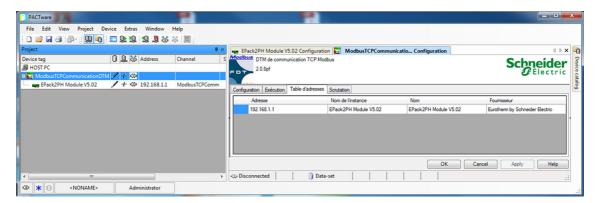
7. Ensure the Project DTM module i.e. (ModbusTCPCommunicationDTM) is selected, select right mouse button and click *Connect*.
