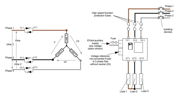
Figure 13 3 phase Star without neutral wiring scheme/load configuration
