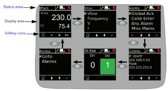
Figure 16 Operator interface
