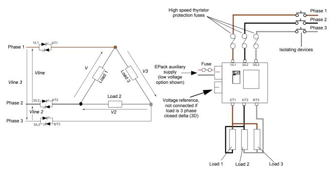
Figure 10 3 phase Closed Delta wiring scheme/load configuration
