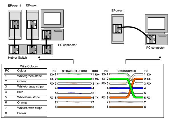
Figure 22 Ethernet (Modbus TCP) Wiring - Single and Multiple EPower controller Units
