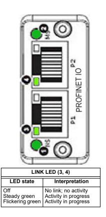
Figure 15 PROFINET connector, double port version
