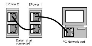
Figure 34 Ethernet/IP Wiring - Multiple EPower controller Units (Single port left, Double port right)
