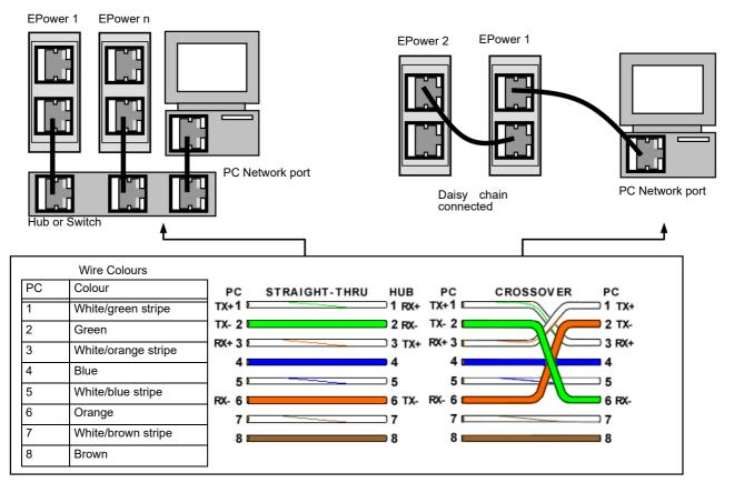
Figure 24 Ethernet (Modbus TCP), dual port – Wiring, Single and Multiple EPower controller Units
