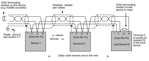
\* On some devices a terminal may be supplied for connection of the shield. Omit this link if the terminal is not available.
