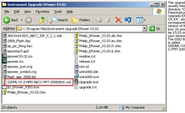
The upgrade tool is usually installed in the directory "C:\Program Files\Instrument Upgrade EPower VX.XX", where X.XX corresponds to current version of the upgrade tool. (In practice this will be V3.03 or newer for your device). The GSD file for EPower is called GSDML-V2.2-HMS-ABC C-PRT-20090618.xml
