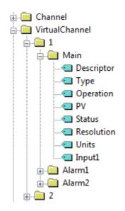
We want to drag the tag called Input1 over to the Input1 field of the Implicit Inputs. Likewise, we will do the same for Virtual Channel 2
