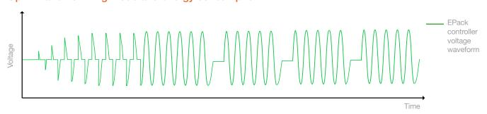
The EPack power controller automatically switches from phase angle to burst firing mode depending upon the ohmic value of the load, for example, during the period of stress when the load is cold. The advanced start-up feature allows smooth start-up with less stress on the load.
