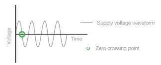
The EPack Controller can accurately detect a zero crossing on the voltage waveform and is able to trigger the thyristor at that moment. This results in less harmonic distortion and RFI, reduction of the dc component, and accurate response to the power demand.
