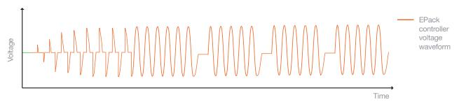
The EPack power controller automatically switches from phase angle to burst firing mode depending upon the ohmic value of the load, for example, during the period of stress when the load is cold. The advanced start-up feature allows smooth start-up with less stress on the load.
