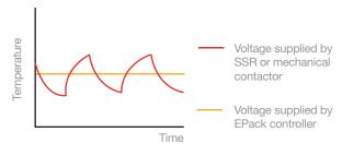
Compared to a standard SSR or mechanical contactor, the EPack Controller adjusts the energy delivered to the heating element, reducing temperature fluctuation and helping to extend the life of the heater.
