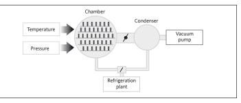
Temperature can either be controlled electrically using heating mats on the shelves, or by circulating oil through pipes welded to the shelves in the chamber. The temperature of the chamber, shelves (and/or heating oil), plus condenser form part of the control and monitoring variables.
