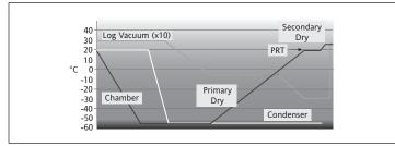
The critical phase is the heating phase where the rate at which the water boils off must be slow enough not to damage the product. During this phase, the vacuum is held constant to give consistent conditions. The temperature ramp has to be held if the vacuum rises too much, indicating that the water is coming off too fast.
