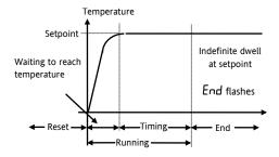
This is the same as mode 1 except that at the end of the timing period the controller will continue indefinitely in automatic control.
