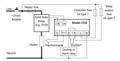
\* When switching inductive loads such as contactors or solenoid valves, wire the 22nF/100 $\Omega$  'snubber' supplied across relay terminals AA & AB. This will prolong contact life and reduce interference.
