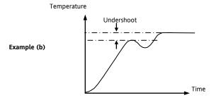
When the temperature approaches the setpoint from above, you can set  $H \subset b$  in a similar manner.
