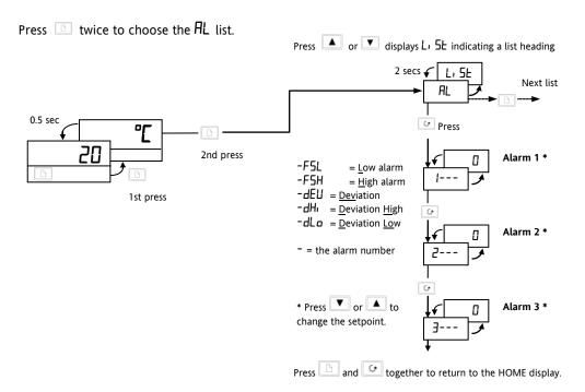
There are three Alarms. The setpoint for each alarm is found under the  $\mathcal{H}_{L}$  list. If an alarm has been disabled, it will not appear in this list.
