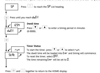
The SEAE parameter can also be switched between OFF and run by configuring the logic I/O as a Off/run contact closure input
