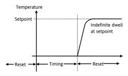
This mode applies a time delay before turning on the heating (or cooling). When the timer is started, the controller will always switch to standby mode and start counting down. When the timer has timed out, the controller will switch into automatic control, apply heating (or cooling) and control indefinitely at the setpoint.
