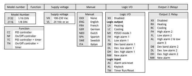
Indicators are supplied configured according to the ordering code shown below:-
