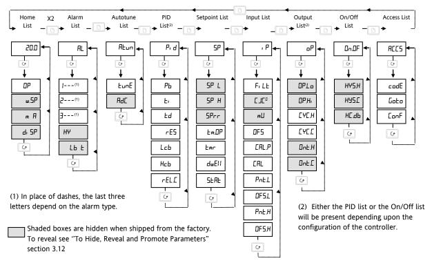
The above diagram shows parameters for a controller. For indicators the Autotune, PID, Output and On/Off Lists are not available.
