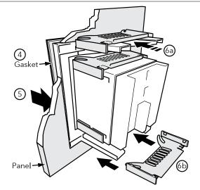
Figure 1b Installing the adapter plate into the panel
