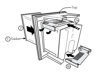
Figure 1a Installing the nanodac into the adapter plate
