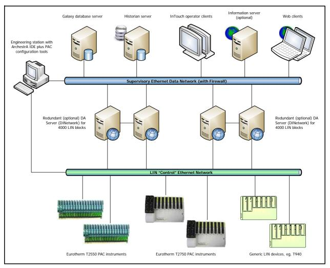
The top half of the figure shows a standard ArchestrA configuration connected to the supervisory network. Connected to this network is:
