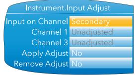
Only those channels with 'Type' set to 'Dual mA', 'Dual mV' or 'Dual T/C' appear in the list of secondary channels. In this example only channels 1 and 3 are configured as dual input.
