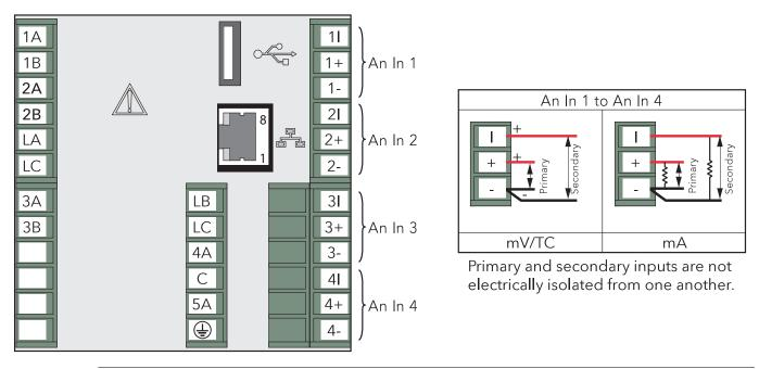
Note: For maximum accuracy, it is recommended that separate returns are used to the negative terminals.
