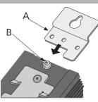
For Bulkhead mounting, fit the upper bracket 'A' to the rear of the unit by removing screw 'B' and associated shakeproof washer, offering the bracket up to the unit, and then securing it using screw 'B' ensuring that the bracket is correctly oriented (as shown) and that the shakeproof washer is fitted between the screw head and the bracket. The relevant screwdriver should have a 3mm
