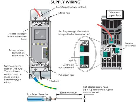
Screwdriver/Torque wrench screwdriver bit details for line and load termination
