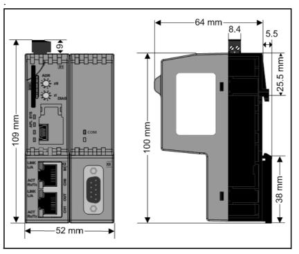
The netHOSTs are typically mounted beside the T2750, and the total width of a T2750 and two netHOSTs fit comfortably within the gap created by the removal of a T940(X). However, it is not necessary to mount the netHOST in close proximity to the T2750, as communication between the two devices is performed using standard 100Mbps Ethernet.
