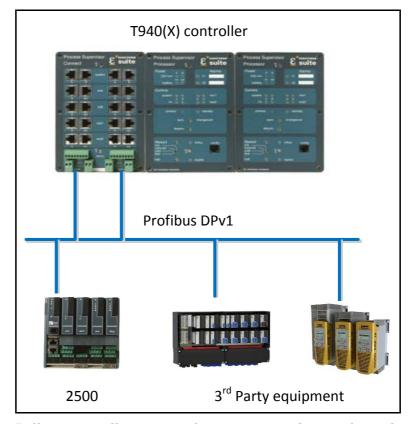
Different installations may have a varying degree of complexity, with or without Profibus requirements, or perhaps using Modbus. Typically, the system is controlled by one or more T940(X) process controllers, and have one or more items of equipment connected to the controller - often over Profibus or Modbus - but sometimes with other protocols. In the example installation above, the T940(X) communicates using the Profibus protocol via its internal Profibus gateway cards.
