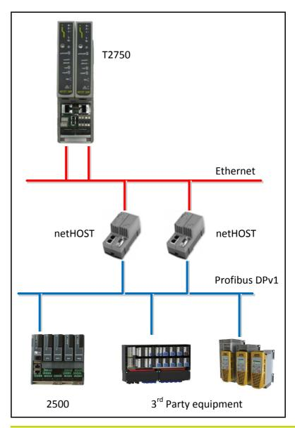
**Note:** The T2750/netHOST combination uses standard 9-pin D-connectors to connect to the Profibus network.
