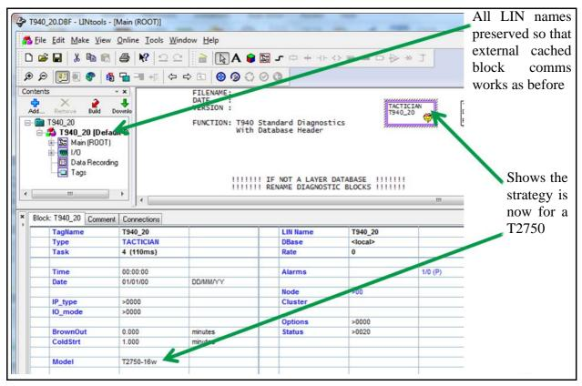
Having completed a migration, the new T2750-version of the database can be downloaded to a T2750 instrument when/if one is attached.
