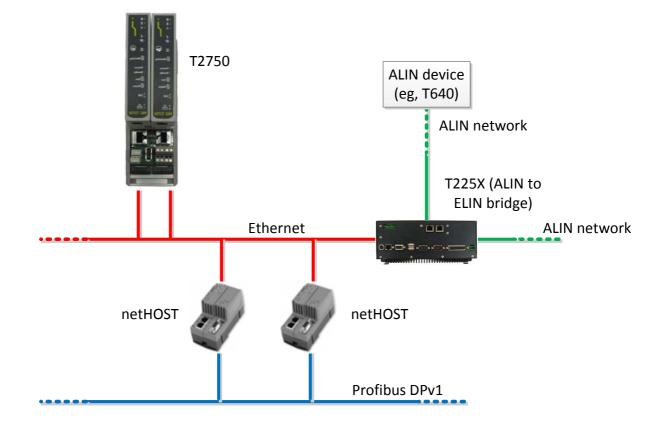
If migrating from an ALIN T940 controller, an ALIN to ELIN bridge is required, as shown in the following figure.
