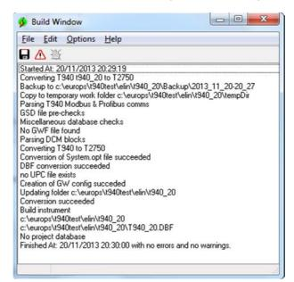
8 If the migration completed successfully, the current loaded database shown in LINTools is the new T2750 version, with a correct Tactician header block (rather than the T940 header block) and appropriate DCM blocks.
