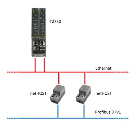
The above figure shows a typical Ethernet network connecting each netHOST to it's corresponding T2750 processor card. A total of four network feeds would be required for this setup.
