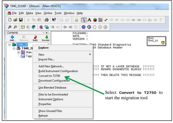
**3** Right-click on the instrument, and select **Convert to T2750** (see figure below).
