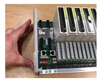
7. If the CPU modules were originally installed, push these back onto the CPU terminal units and lock in place with the screwdriver. Reattach the front cover to the hinges.
