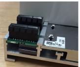
6. Push the end panel back on by hand, ensuring it is aligned with the chassis.
