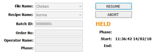
Figure 10 HMI Control Panel (file held)
