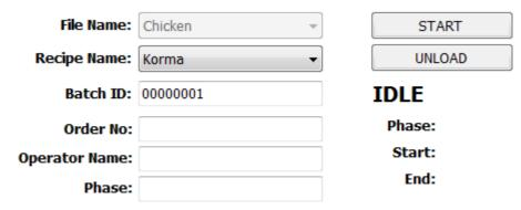
Figure 8 HMI Control Panel (file loaded - ready to start)
