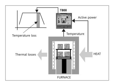
Eurotherm have created a modelling algorithm which calculates an oven parameter, allowing the temperature uniformity of a load to be defined. This then allows the cycle time, regardless of the load, to be optimised.
