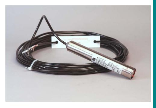
Level transmitter with submersible probe in stainless steel for applications where pressure connection in the bottom is not possible or desirable. E.g. pump pits, reservoirs or plastic tanks.
