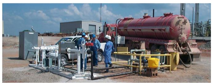
Truck Unloading: Multi-phase flowmeter accurately measures barrels of net oil regardless of trapped air content without need of an air eliminator
