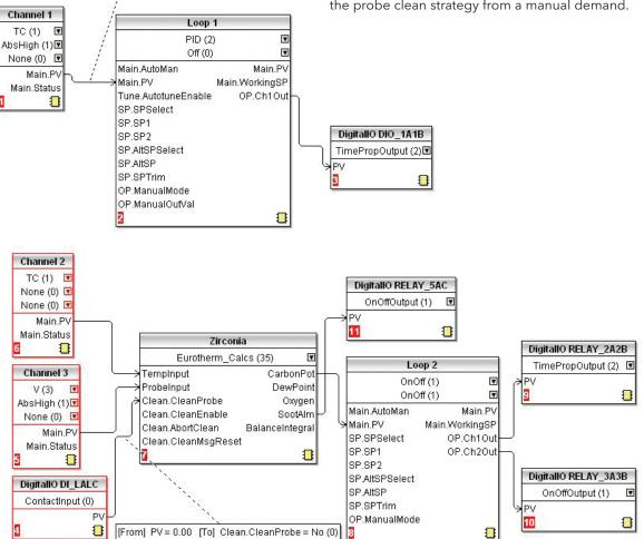
Graphical View of 'Soft' Wiring using iTools
