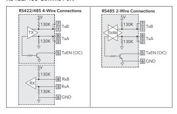
The PGX-RS option card has one RS422/485 port. This port can be configured to act as either RS422 or RS485.
