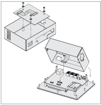
CAUTION - THE OPTION AND MAIN CIRCUIT BOARDS CONTAIN STATIC SENSITIVE COMPONENTS. BEFORE HANDLING THE CARDS, DISCHARGE STATIC CHARGES FROM YOUR BODY BY TOUCHING A GROUNDED BARE METAL OBJECT. IDEALLY, HANDLE THE CARDS AT A STATIC CONTROLLED CLEAN WORKSTATION. ALSO, HANDLE THE CARDS BY THE EDGES ONLY. DIRT, OIL, OR OTHER CONTAMINANTS THAT MAY CONTACT THE CARDS CAN ADVERSELY AFFECT CIRCUIT OPERATION.
