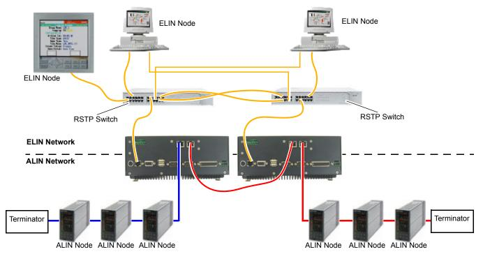
Figure 2-1: Wiring examples
