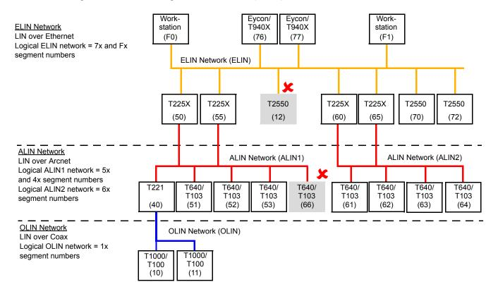
Note The rules previously described apply to all Bridge units, including the T225X, T225, T221 and the NTSE when configured as a Bridge unit.
