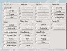
The InTouch HMI also empowers users to quickly and easily develop custom graphical views of their processes. A user can develop graphics with a variety of tools in Wonderware's WindowMaker™ graphical editing program, which includes standard graphical components, bitmap images, ActiveX®
