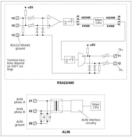
Figure 2-9 T640 communications zero volts schematic
