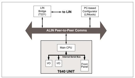
Figure 7-2 ALIN communications schematic
