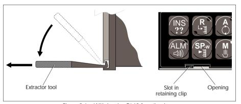
Figure 2-4 Withdrawing T640 from the sleeve
