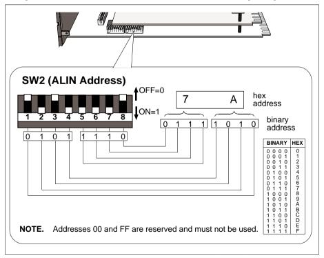
Figure 2-13 SW2 — ALIN address setup (example)
