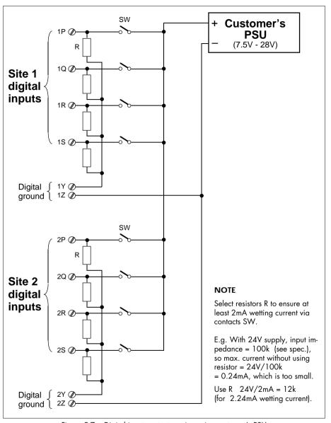
Figure 9-7 Digital input contact-sensing using customer's PSU
