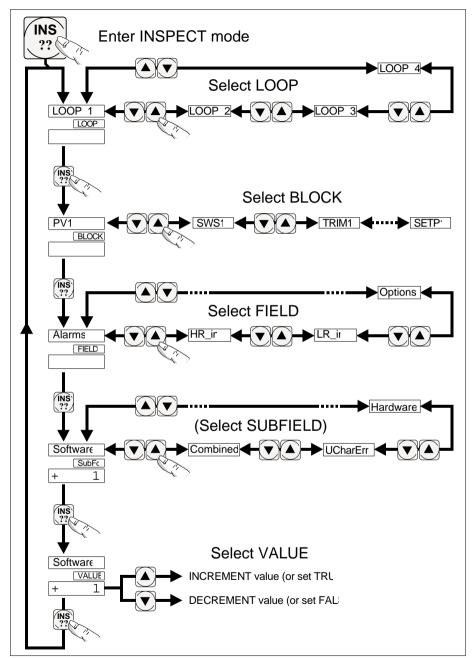
Figure 4-2 Inspect button functions — INS
