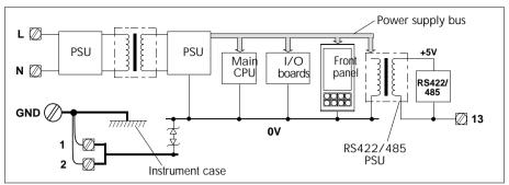
Figure 2-7 T640 internal zero volts & power supplies schematic
