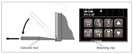
Figure 3-3 Removal of T640 from sleeve
