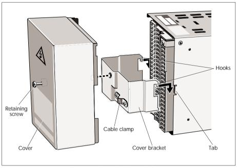
Figure 2-5 Removing the terminal cover
