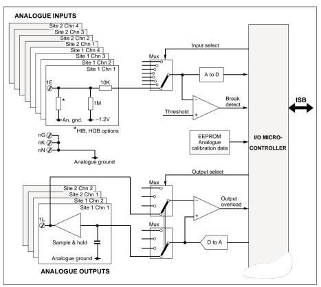
Figure 9-2 Analogue input & output block schematic
