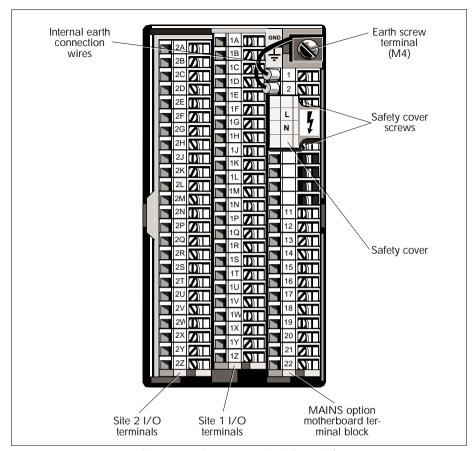
Figure 2-6 Customer terminals (example)
