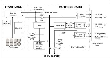
Figure 7-1 T640 Functional block schematic
