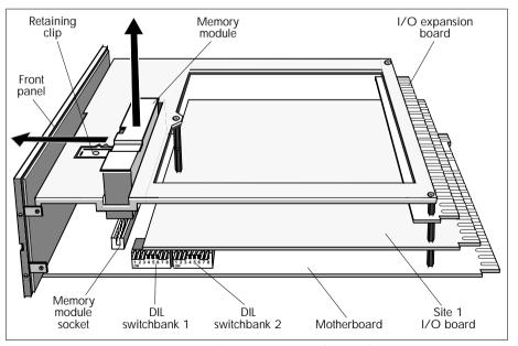
Figure 2-10 T640 internal layout (example)
