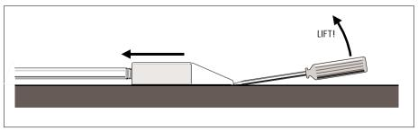
Figure 2-3 Removing a clamp from the sleeve
