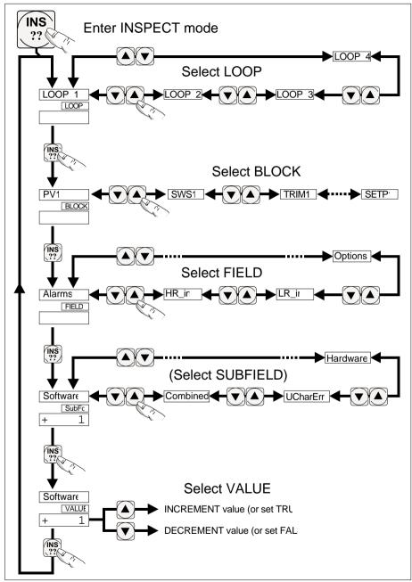
Figure 3-10 Inspect button functions — INS
