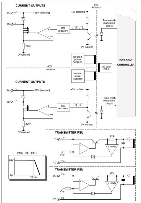
Figure 9-4 Current output & transmitter PSU block schematic
