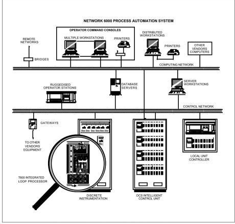
Figure 1-1 Network 6000 distributed control system
