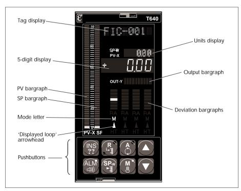
Figure 3-7 T640 front panel — initial power up
