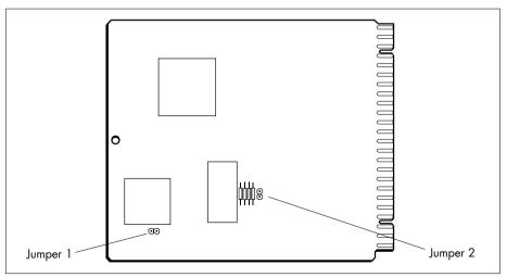
Figure 9-1 High-level I/O board showing 0 - 1.25V range jumpers
