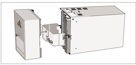
Figure 3-1 Terminal cover removal
