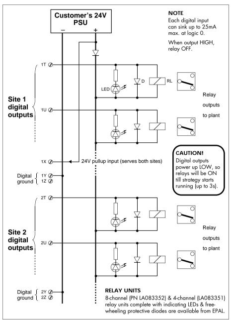
Figure 9-6 Digital outputs operating relays (current sinks) with pullup via customer's PSU
