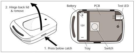
Figure 4-5 Security key — battery replacement
