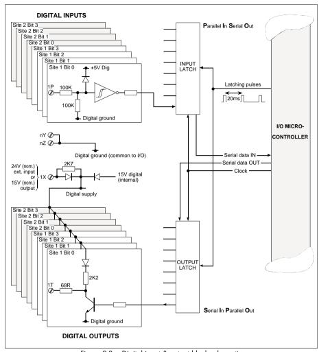
Figure 9-3 Digital input & output block schematic
