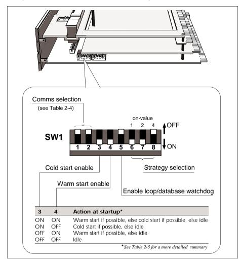
Figure 2-12 SW1 location and functions
