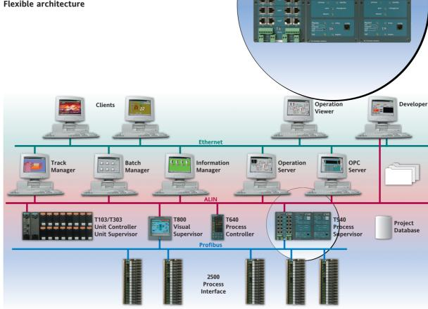
The Process Supervisor is a powerful and configurable strategy engine capable of performing both continuous and sequential control. It has evolved from the successful T103/T102/T100 Unit Controllers and is designed for large applications.
