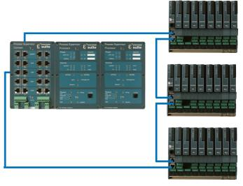
In duplex operation, the two processor modules are designated one as primary and the other as secondary. On power-up the primary module runs the control strategy and communications while the secondary tracks the primary operation and status via a high-speed data link. Upon detection of a failure in the primary processor, the changeover form the primary to the secondary will be automatic and bumpless, initiated by watchdog circuits and software checks.
