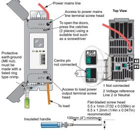
Screwdriver/Torque wrench screwdriver bit details for line and load termination
