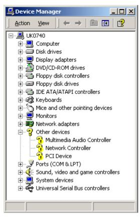
The detected Arcnet card appears in the Other devices folder with the default name 'Network Controller'.
