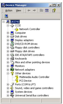
The installed Arcnet card appears in the CCSI folder with the default name 'Network Controller'.
