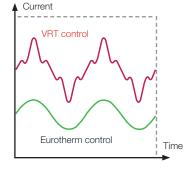
Eurotherm digital thyristor power control helps to provide linear control across the entire output % range, whereas the VRTs cause unstable control at low setpoints.
