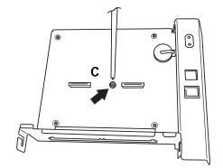
Figure 2.3 Remove securing screw
