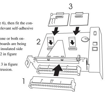
Figure 4.8 Fit connector, flexi cable(s) and option board(s)
