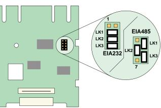
Figure 4.3 Serial communications board: selection of transmission standard
