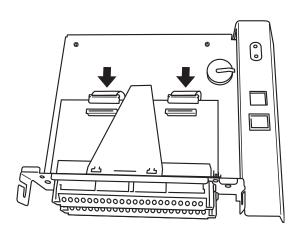
Figure 4.9 Make the flexi cable connections
