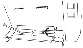
Figure 3.1 Remove blanking plates
