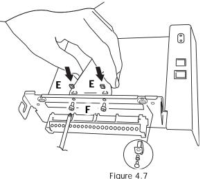
Fit the board guide extrusion and EMC spring (if required)
