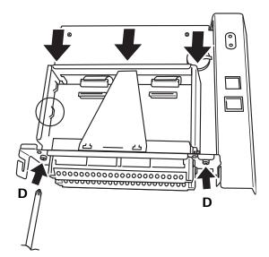
Figure 4.10 Fit the board support bracket
