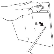
Figure 2.2 Remove securing screw
