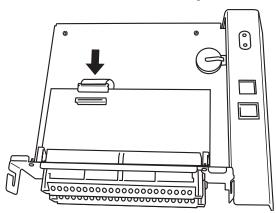
Figure 3.5 Make the flexi cable connection
