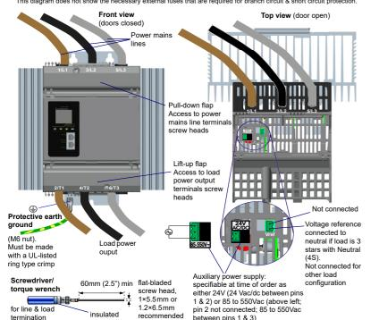
A 63A EPack is shown below. Units for other current ratings are of similar appearance and are wired in the same manner. Use a 0.6 × 3.5 mm screwdriver for pluggable connectors
